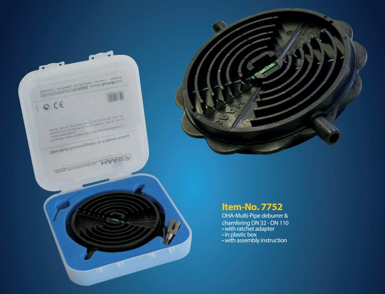
For deburring and chamfering the inner and outer edges in one operation. Ground and hardened cutting blade for extra long life, made of sturdy plastic for low abrasion and long life. Suitable for HT, KG Geberit<sup>®</sup> Silent-PP, Valsir<sup>®</sup> HD-PE, POLO-KAL<sup>®</sup> NG Pipes in DN 32, DN 40, DN 50, DN 56, DN 60-63, DN 70-75, DN 90 and DN 100-110. Accessories: Adapter? For ratchet: Art.-No . 7753 and knife change kit: Art.-No . 7754
