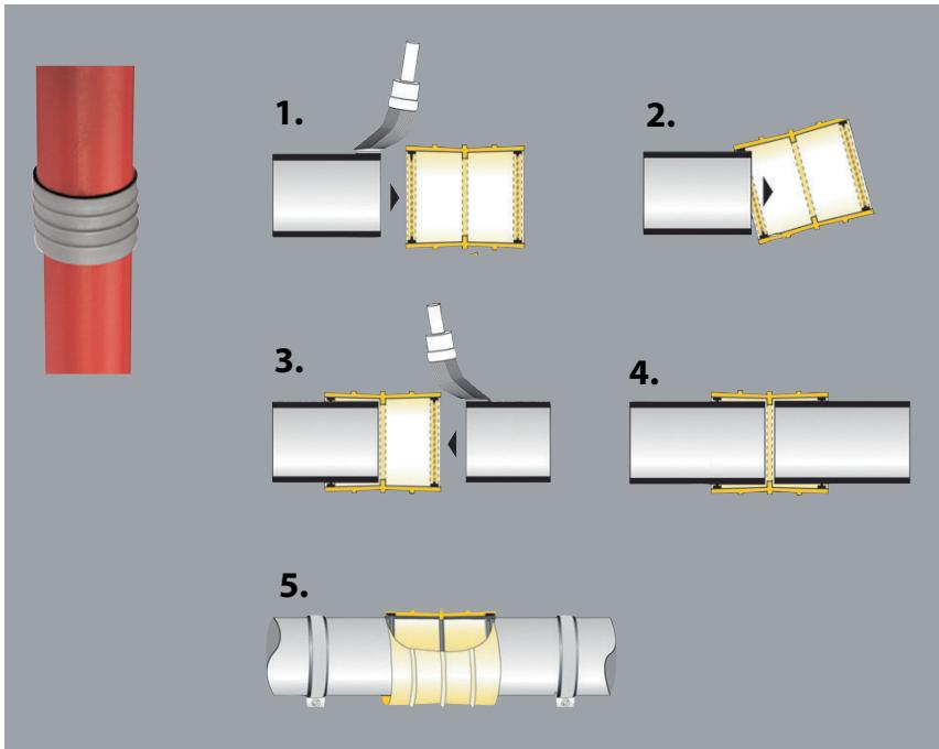
Plug-in connector for cast iron/TML/BML pipes in the field of property drainage and house drainage pipes. Manufactured according to official construction and testing specifications. Double socket made of PP in gray color with directly molded lip seals made of TPE. Easy, safe installation, as no slipping of the seal is possible. When using the SVE connector inside buildings, we recommend to additionally secure the pipes and fittings if necessary due to the elasticity of the connection.
