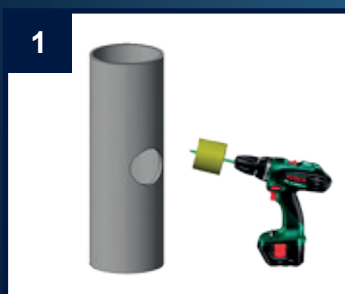
1. Drill the hole \varnothing 57 mm
