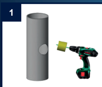
1. Drill the hole \varnothing 57 mm
