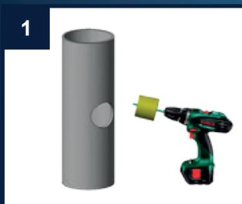
1. Loch bohren Ø 57 mm
