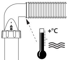
2. Releasing of the junction between angle and hose
